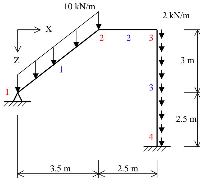
Member properties are; member 1 & 2:  $A: 0.08 \text{ m}^2$   $I_y: 1.067 \cdot 10^{-3} \text{ m}^4$   $E: 3 \cdot 10^7 \text{ kN/m}^2$ , member 3:  $A: 0.15 \text{ m}^2$   $I_y: 2.0 \cdot 10^{-3} \text{ m}^4$   $E: 2 \cdot 10^8 \text{ kN/m}^2$ .
