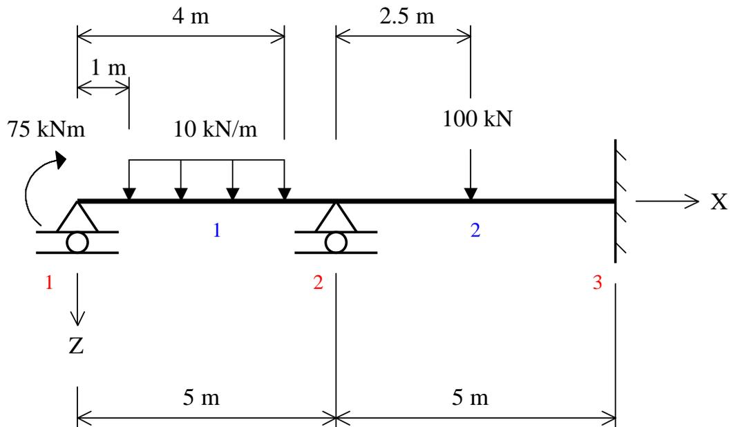
The properties of member 1 & 2 are:  $A: 0.08 \text{ m}^2$   $I_y: 1.067 \cdot 10^{-3} \text{ m}^4$   $E: 3 \cdot 10^7 \text{ kN/m}^2$
