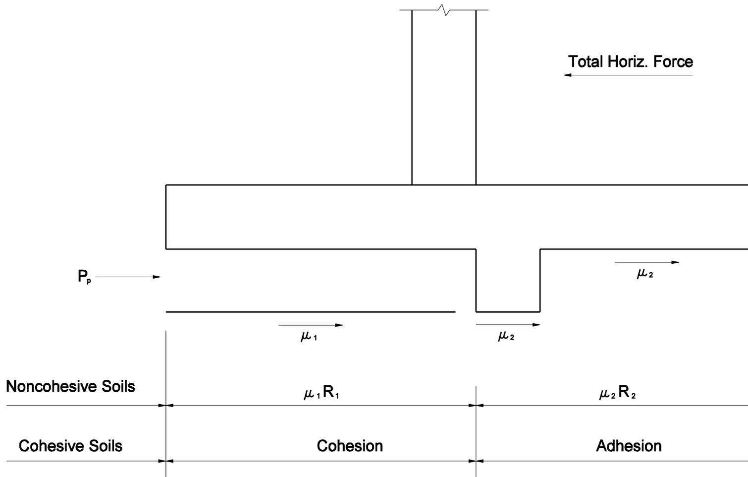
$\mu_1$  = Coefficient of friction for soil on soil
