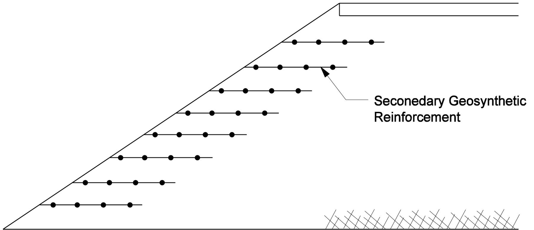
**SLOPE REINFORCEMENT PROVIDING LATERAL
