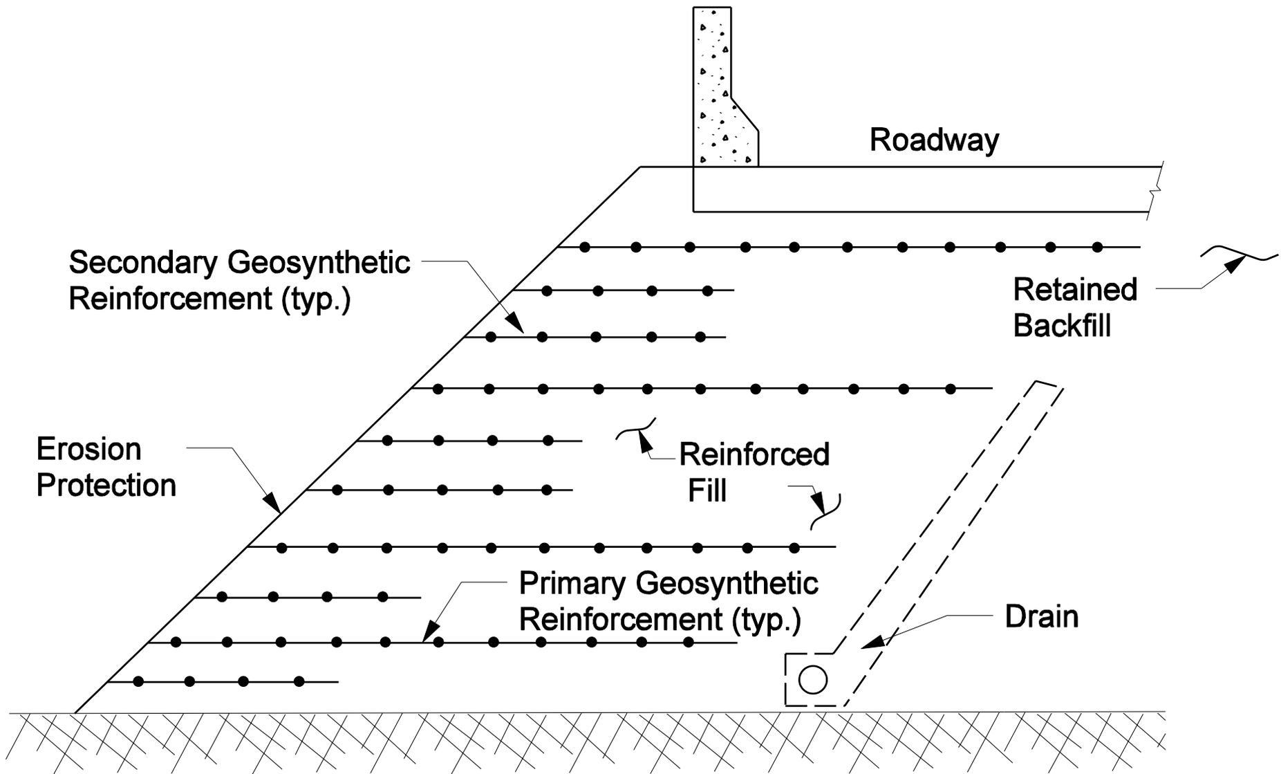
**SLOPE REINFORCEMENT USING GEOSYNTHETICS
