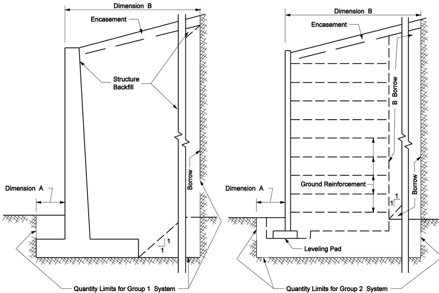
**Note:** The limits for establishing pay quantities for alternate wall designs should be identical. The outermost limit of construction for any individual wall should be used as the limit for computing pay quantities for all other alternate wall designs.
