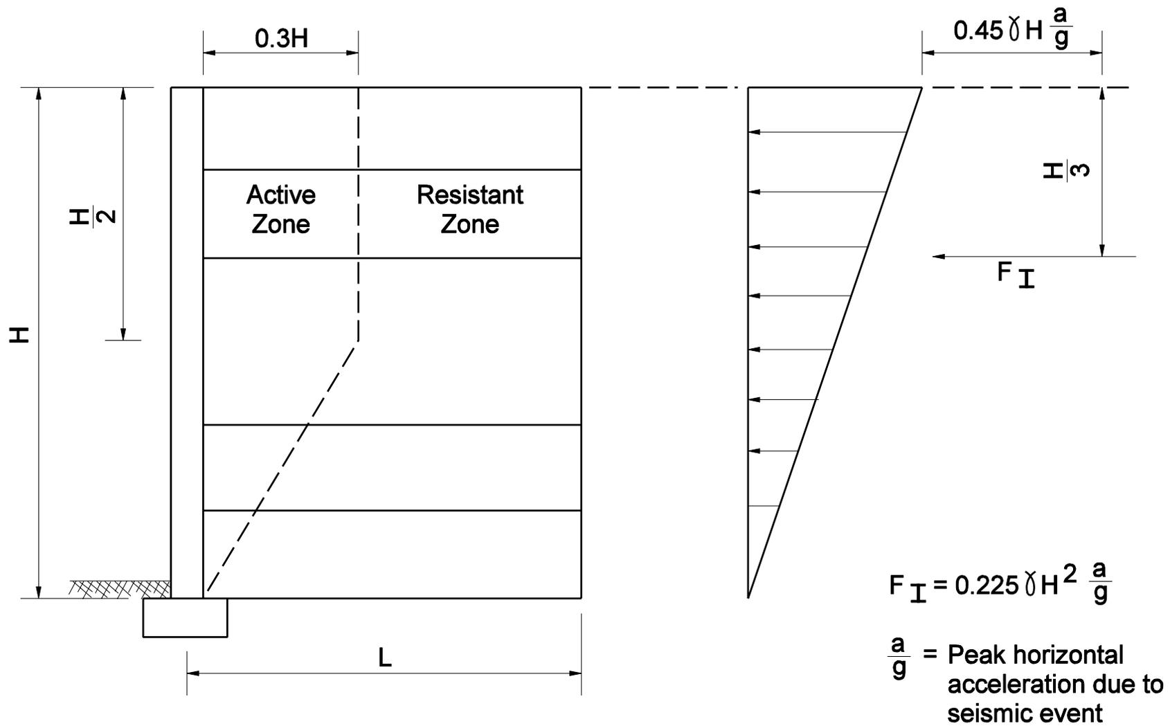
INERTIAL SEISMIC FORCE DISTRIBUTION,
